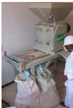
Fig. 2 Two roll roller mill used to produce roller milled meal samples.
