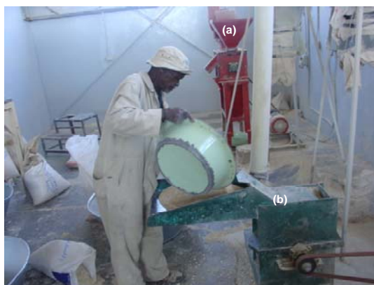
Fig. 1 PRL-type Abrasive decorticator (a) and hammer mill (b) similar to those used to produce abrasive decortication-hammer mill meal samples.
