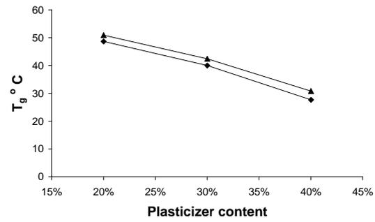
**Figure 2.** T<sub>g</sub> of prolamin films with different plasticizer contents.
