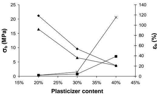
**Figure 3.** Stress at break and strain at break of prolamin films with different plasticizer contents.
