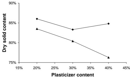
**Figure 1.** Dry solid content (w/w) of prolamin films with different plasticizer contents.
