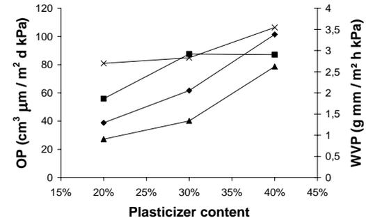
**Figure 4.** Barrier properties of films with different plasticizer contents.
